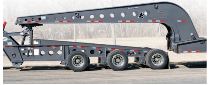
24" vertical travel hydraulic Power Tower. Lifts full load.
