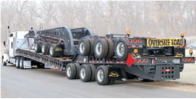
Stackable 53' O.A.L. under 80,000# gross (depends on truck weight and deck length).
