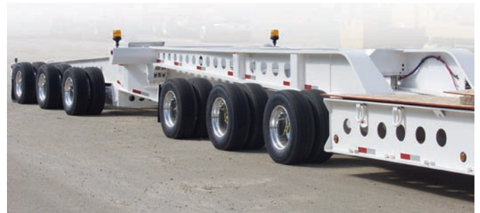
West coast walking beam suspension for travel over uneven terrain.
