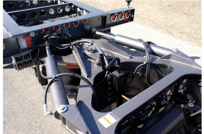
Hydraulic bump steering for backing trailer.
