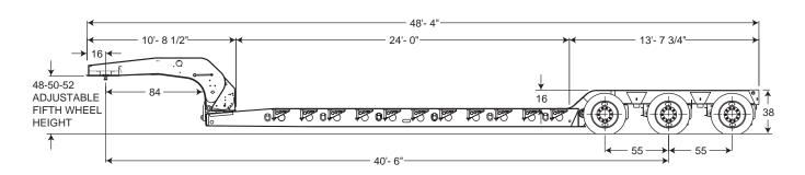
**General:** 50/55 ton capacity, three axle, non-ground engaging hydraulic
