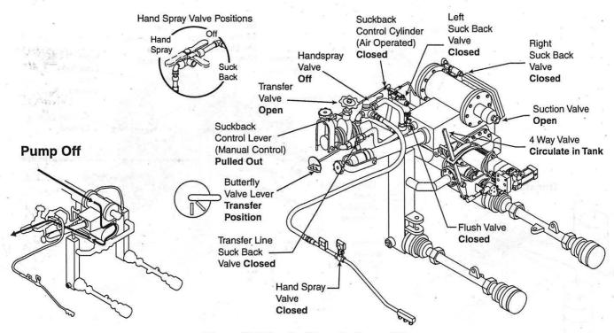
Figure 13. Valve Positions for Pump Off
