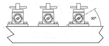
Figure 7. Adjusting the Spray Bar Nozzles
