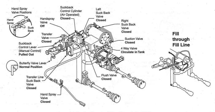
Figure 3. Valve Positions for Filling Through the Fill Line
