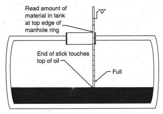
Figure 2 Using the Measuring Stick
