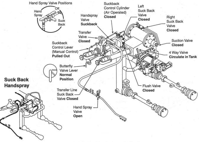
Figure 12 Valve Positions for Handspray Suckback
