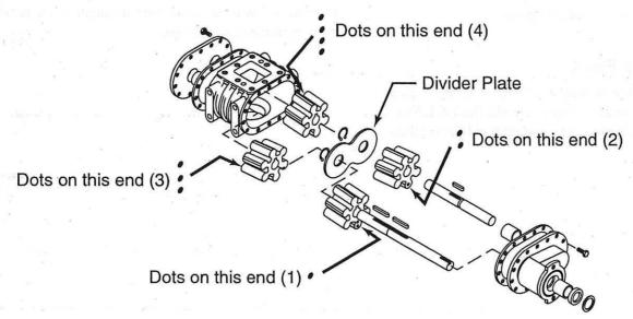
Figure 24 Etnyre Asphalt Pump
