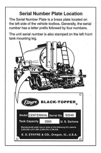
Figure 26 Serial Number Plate Location
