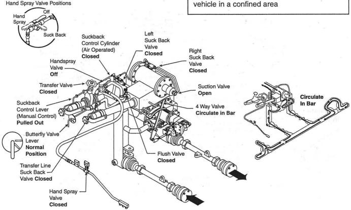
Figure 6. Valve Positions for Circulating in the Bar
