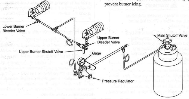
Figure 16. Manual Control Burner System
