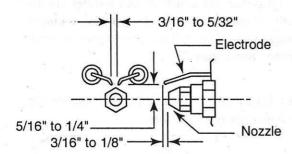
Figure 20. Burner Electrode Adjustments
