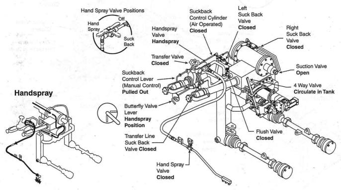
Figure 11. Valve Positions for Handspray.
