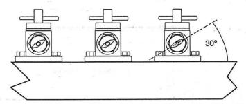
Figure 22. Nozzle Angle Adjustment
