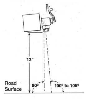
Figure 23 Nozzle Height Adjustment
