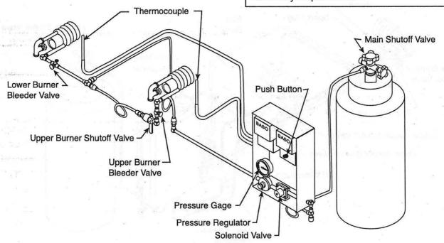
Figure 17. Outfire Controlled Burner System
