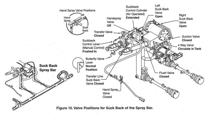
Ensure that the self flush valve is closed at the end of this function, or before loading or circulating asphalt to eliminate chances of inducing asphalt into the self flush fuel tank.
