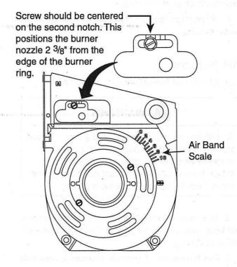
Figure 21a. Nozzle Adjustment
