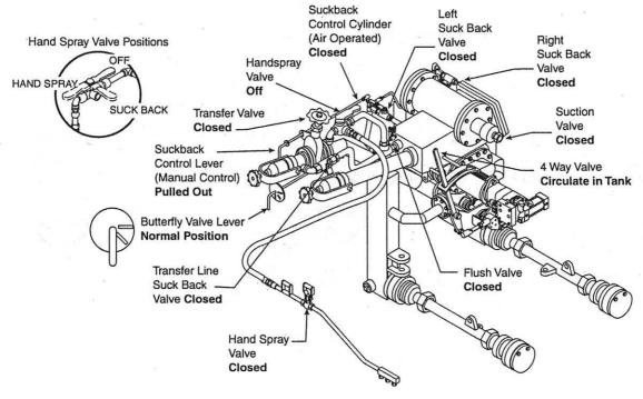
Figure 4. Valve Positions for Filling Through the Manhole
