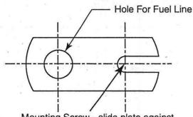
Mounting Screw - slide plate against mounting screw. This will position nozzle in air tube.
