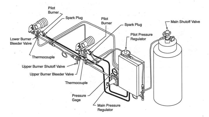
Figure 18 Burner System with Auto Ignition & Temperature Control
