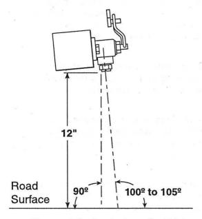
Figure 8. Adjusting the Spray Bar Height.
