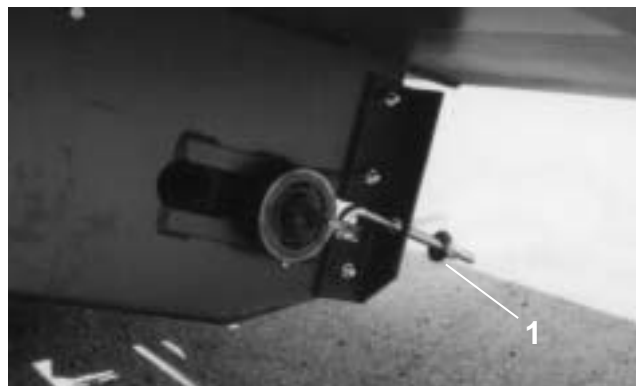
Figure 18. Conveyor Tail Pulley
