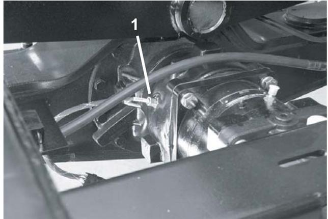
Figure 6. Ground Speed Pickup
