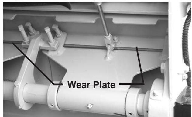
**Figure 14. Hopper Gate Wear Plate**
