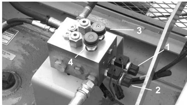
**Figure 11. Belt Speed Controls**
