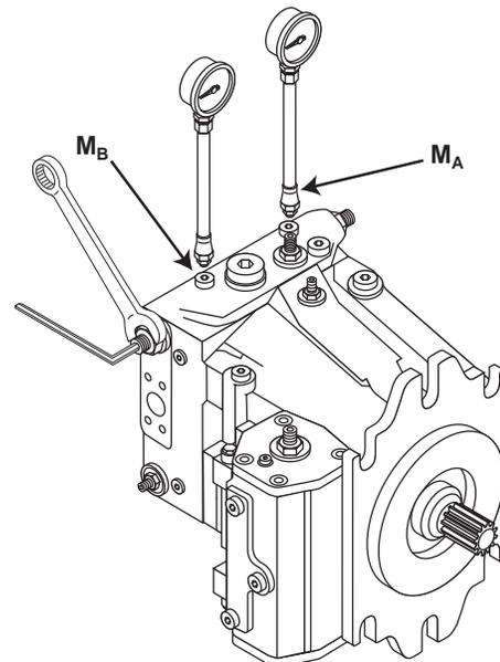
Figure 25. High Pressure Relief Setting
