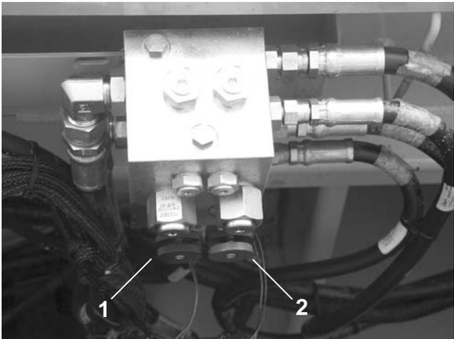
**Figure 29. Right Auger/ Spread Roll Manifold**
