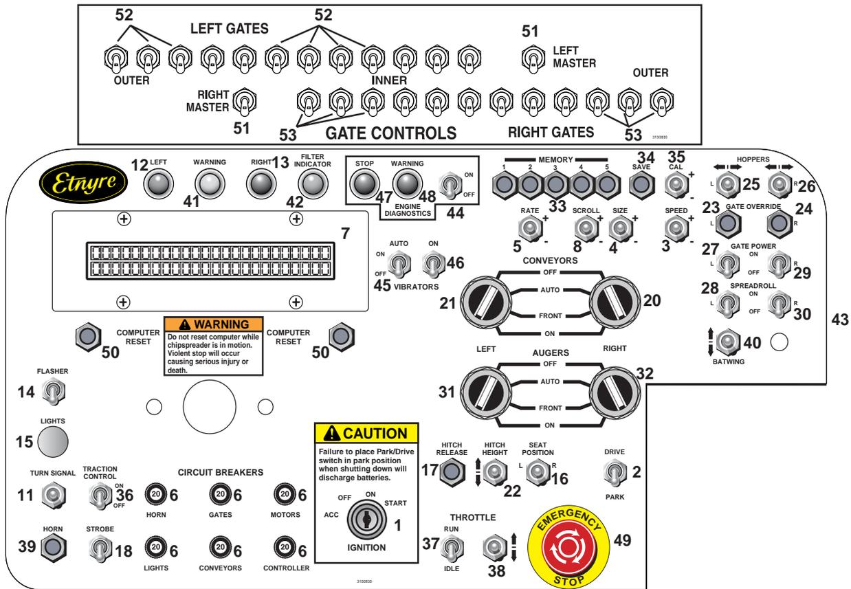
Figure 4. Control Panel Identification
