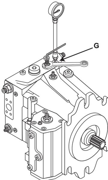
**Figure 26. Charge Pressure Adjustment**
