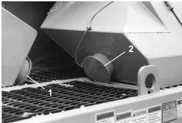
**Figure 10. Conveyor Diaphragm Switches**
