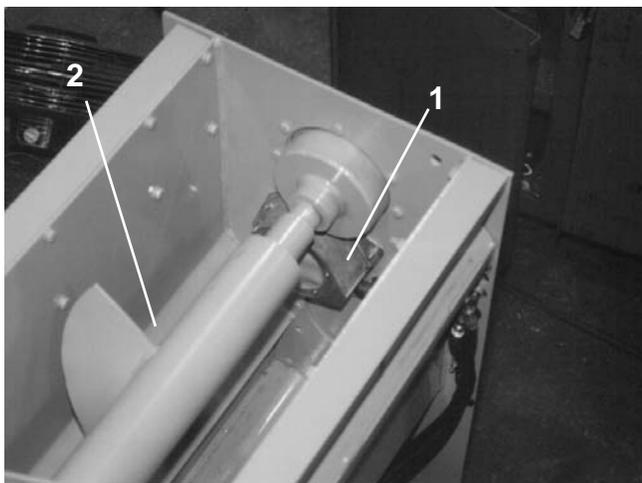
**Figure 8. Auger Auto On/Off Switch**
