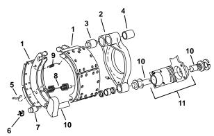
Figure 27. Brake Components
