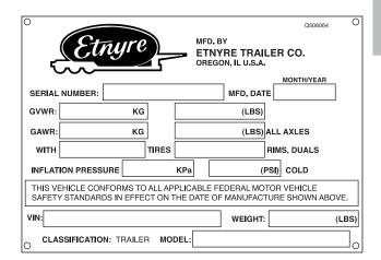
Figure 2. Unit Nameplate or Certification Label
