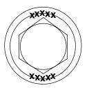
1/4" Fillet Welds, 1" Long, After Axle Is Aligned.
