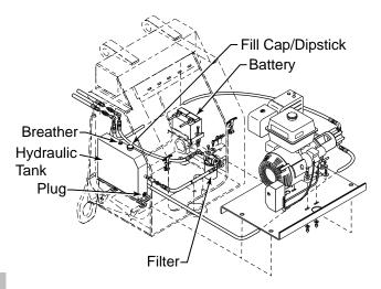
Figure 31. Hydraulic Oil Check
