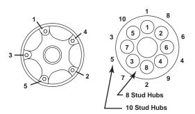
Tighten Lug Nuts to recommended torque using sequence shown
