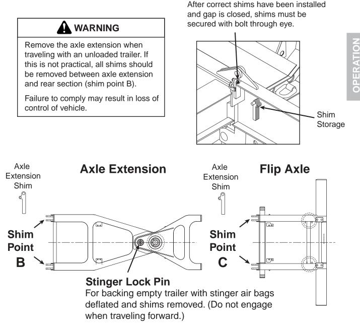
Shim Point **B** for desired load on Stinger Axle. Add shims for more weight on stinger axle, remove shims for less weight on stinger axle. Shim Point **C** for desired load on Stinger Axle. Add shims for more weight on stinger axle, remove shims for less weight on stinger axle.
