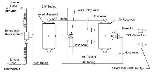
Figure 24. Brake Air Supply System - 2 Axle Shown
