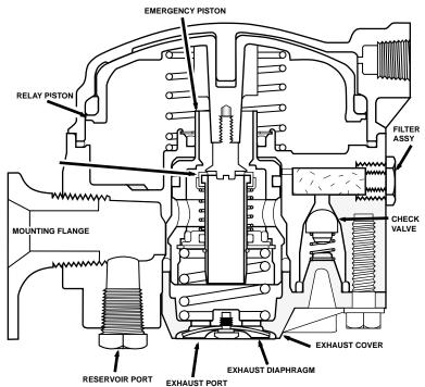
Figure 25. Relay Emergency Valve
