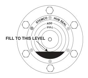
Figure 13. Check Oil Level of Oil Lubricated Bearings.
