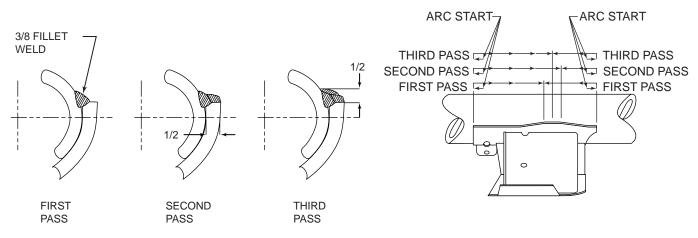
Figure 17. Multiple Pass Recommended Method
