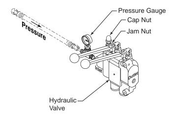
Figure 32. Directional Control Valve Pressure Relief
