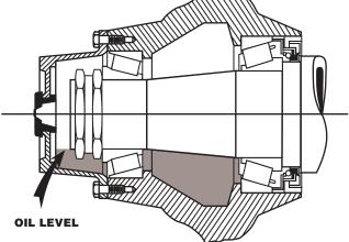
Figure 23. Checking Oil Level in Hub
