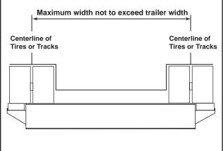
Top of extension bracket boards must be flush with main deck boards.
