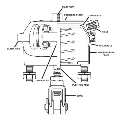
Figure 26. Brake Chamber
