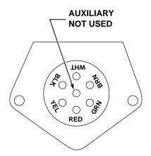
Figure 30. Gooseneck Socket Connection
