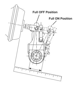
Figure 29. Measuring Maximum Stroke
