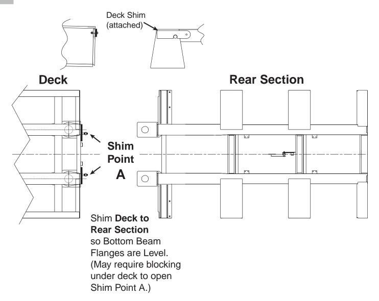
Shimming objective is to have all rear section bottom beam flanges level (top of axle to bottom flange of rear beam should be 6 1/2" at standard ride height). A chart should be kept of all the loads that require shimming and must be developed through trial and error.
