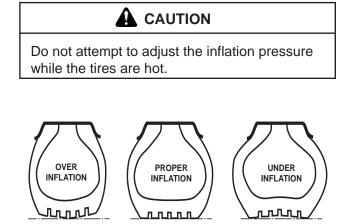
Figure 21. Proper Tire Inflation
