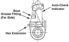
Figure 28. Slack Adjuster Lubrication Points
