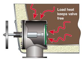
Rear Discharge Valve. 6" valve, complete drainage.
