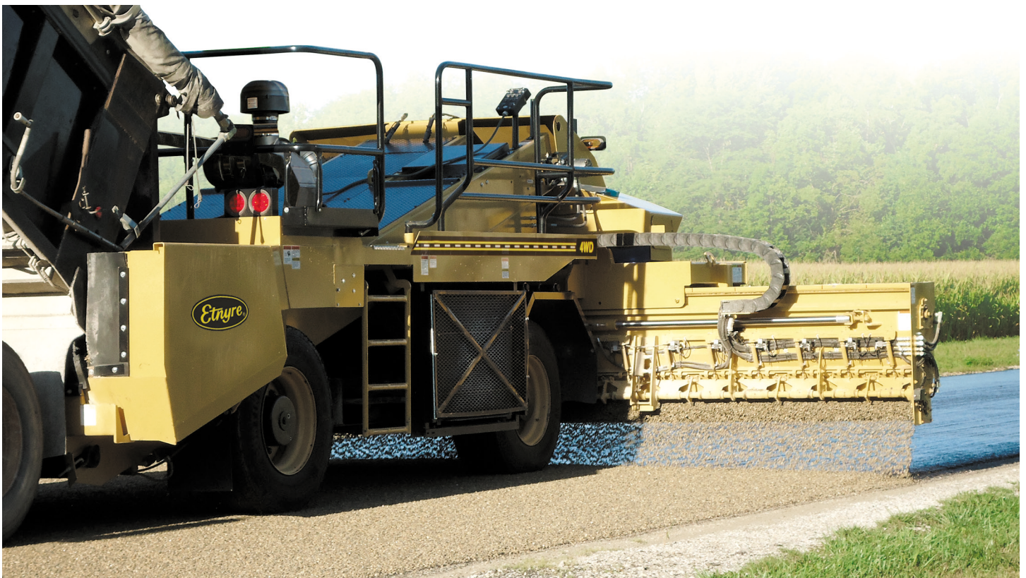
ChipSpreader with four wheel drive and variable width spread hopper
