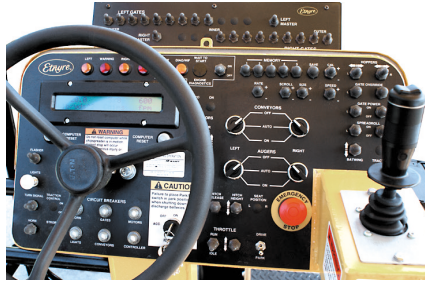
Control Panel provides clear view and easy control. Change from forward to reverse with one hand without clutching.
