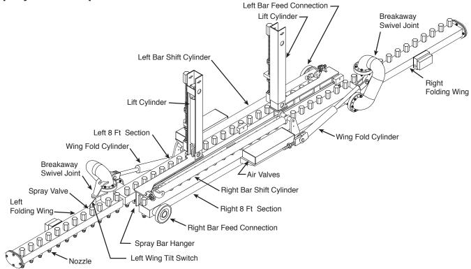
Figure 4. Spray Bar Component Identification
