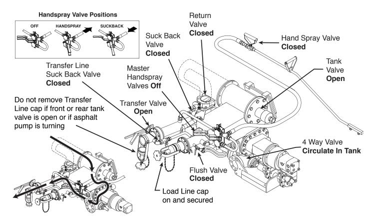
Figure 23. Valve Positions for Unload with Distributor Pump
