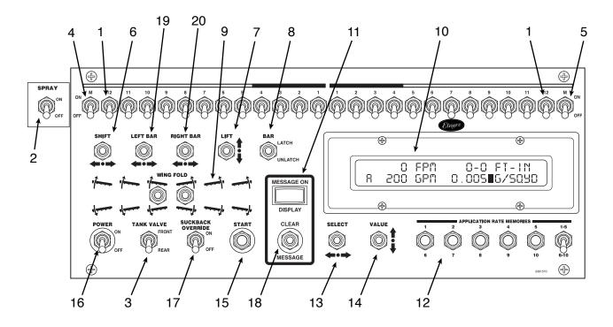
Figure 6. Cab Control Panel Components
