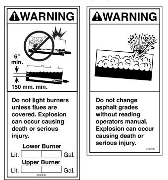
Use the measuring stick as shown in **Figure 12** in the *Using the Measuring Stick* section to determine the amount of product in the tank before lighting burners. The minimum amounts shown on the warning placard only apply if the tank is level.
