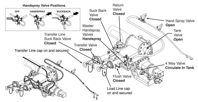
Figure 17. Valve Positions for Handspray
