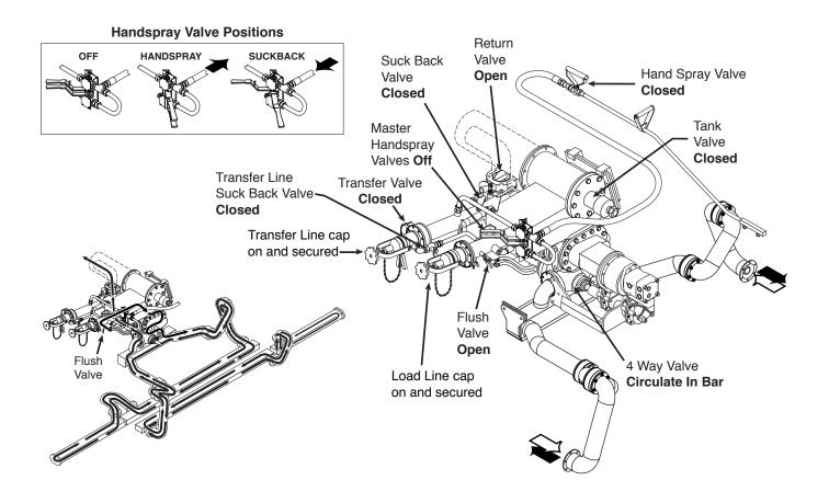
Figure 19. Valve Positions for Flushing
