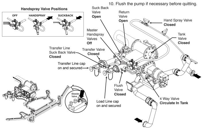
Figure 18. Valve Positions for Spray Bar Suck Back
