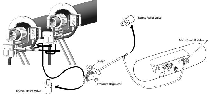
Figure 26. Ignition & Out Fire Control System
