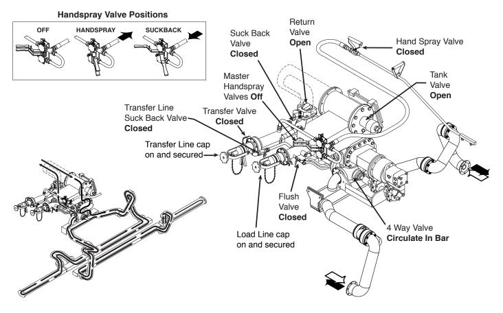
Figure 15. Valve Positions for Circulating in the Bar
