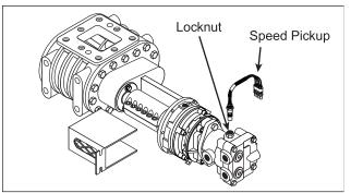
Figure 31. Hydraulic Motor
