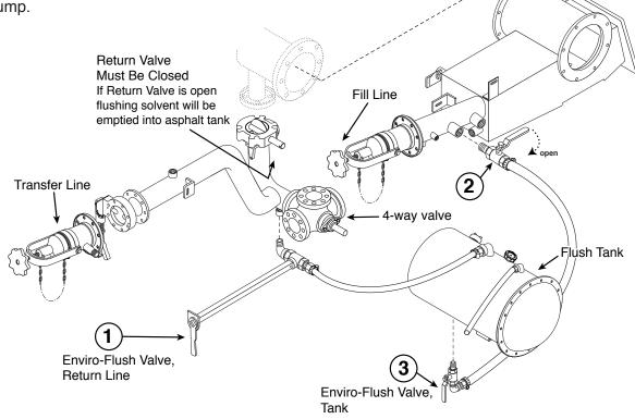
Figure 21. Recirculating Flushing System Operation
