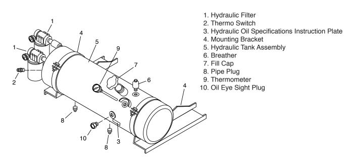
Figure 5. Hydraulic Tank Component Identification
