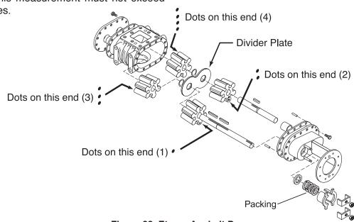
Figure 32. Etnyre Asphalt Pump
