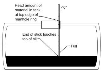
Figure 12. Using the Measuring Stick
