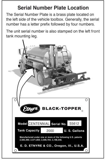
Figure 34. Serial Number Plate Location
