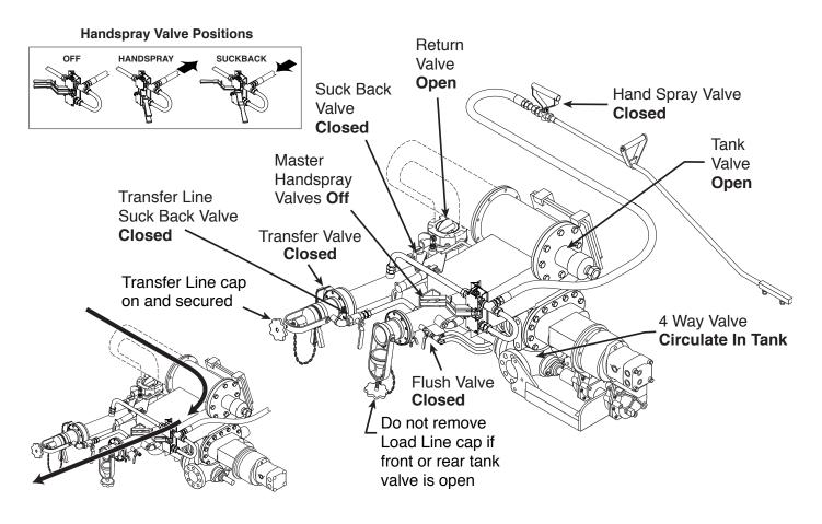
Figure 22. Valve Positions for Unload with External Pump
