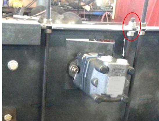
Drive Chain Tension adjustment
