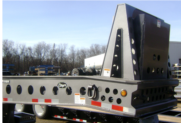
Mechanical Gooseneck with Hydraulic Power Tower
