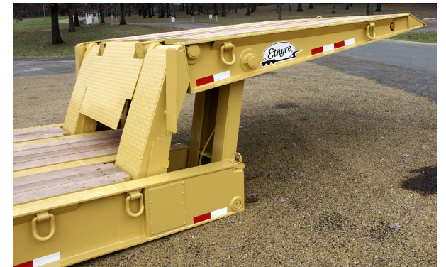
Hydraulic Folding Gooseneck - Knife Nose
