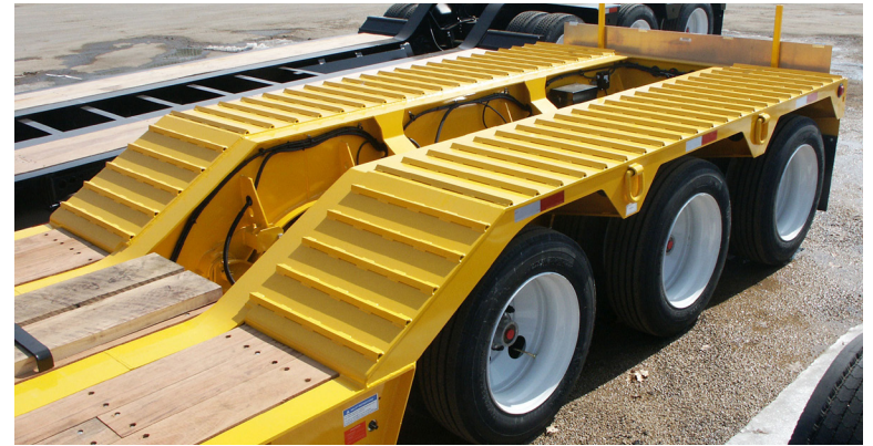
One piece (weld on) with traction bars.
