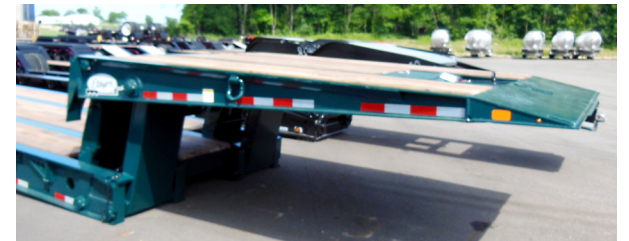
Hydraulic Folding Gooseneck - Tapered Nose
