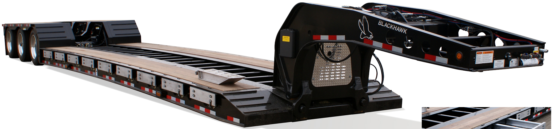
Hydraulic Removable Gooseneck 40 Ton Capacity with pullout deck extensions
