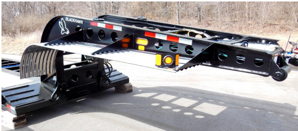
Narrow Mechanical Gooseneck with Fenders
