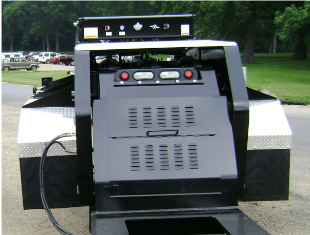
Full Lockable Door with Light Bar and Aluminum Gooseneck Fenders
