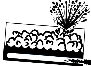
Before lighting burner unLatch manhole to prevent pressure in tank. Explosion can occur causing death or serious
