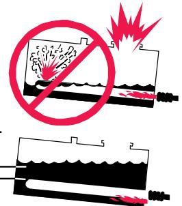
Do not light burners unless flues are covered. Explosion can occur causing death or serious injury.
