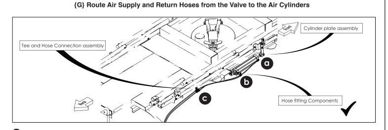
G - Route Air Supply and Return Hoses from the Valve to the Air Cylinders Fixed to Either Side of the Handrails Assembly
