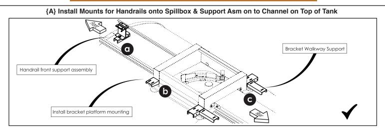
A - Install Mounts for Handrails onto Spillbox & Support Asm on to Channel on Top of Tank
